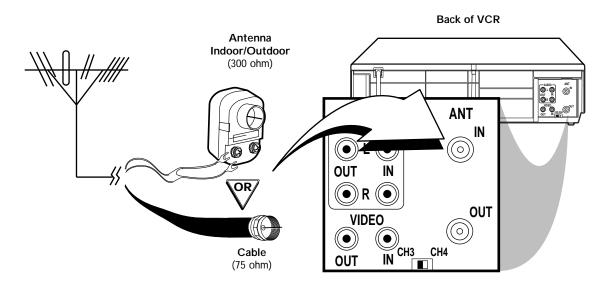
Connect the RF coaxial cable (supplied) to the OUT Jack on the back of the VCR and to the ANTENNA IN Jack on the TV. (You may use either a snap-on type (supplied) or screw-on type of coaxial cable, whichever you prefer.)
